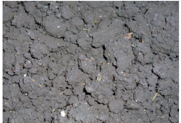
Dewatered sewage sludge with 35 % solids content- no problem for an ABEL solids handling pump
