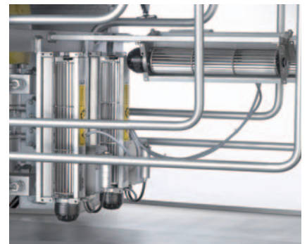
Tangential blowers to cool valve cylinders
