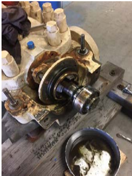
Damaged Thrust Bearing
