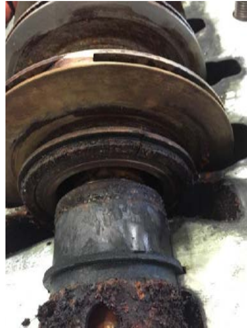
Broken casing wear ring and damaged impeller wear ring
