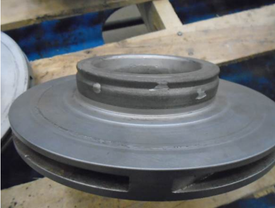
Impeller wear rings are worn.
