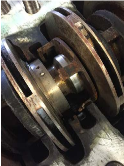
Broken casing wear ring and damaged impeller wear ring
